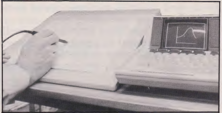
Above: Using the graphics tablet and stylus to input a shape to the HP-83.
